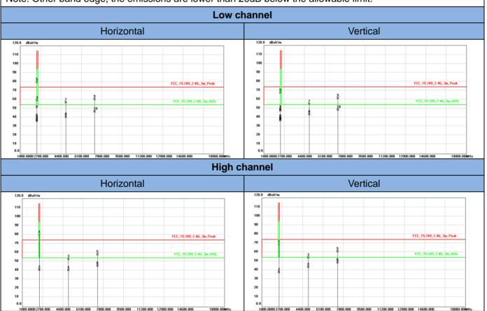
Remark: The emissions for frequency above 18GHz are attenuated 20dB below the limit, it does not record in report.
