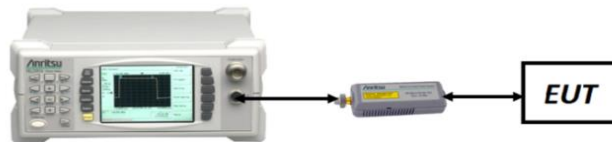
Figure 7-2. Test Instrument & Measurement Setup
