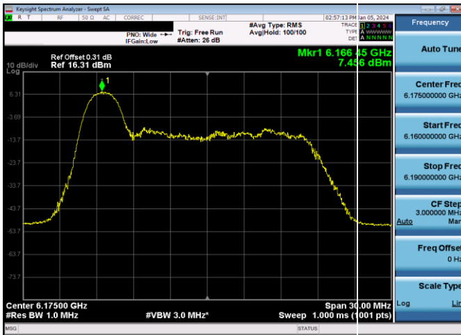
Plot 7-129. SP Power Spectral Density Plot Antenna WF8 (20MHz 802.11ax RU26 (UNII Band 5) – Ch. 45)
