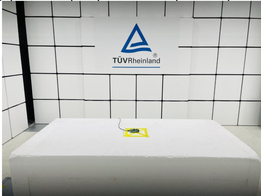
Photograph 2: Test Setup for Spurious Emissions (Front View 2)
