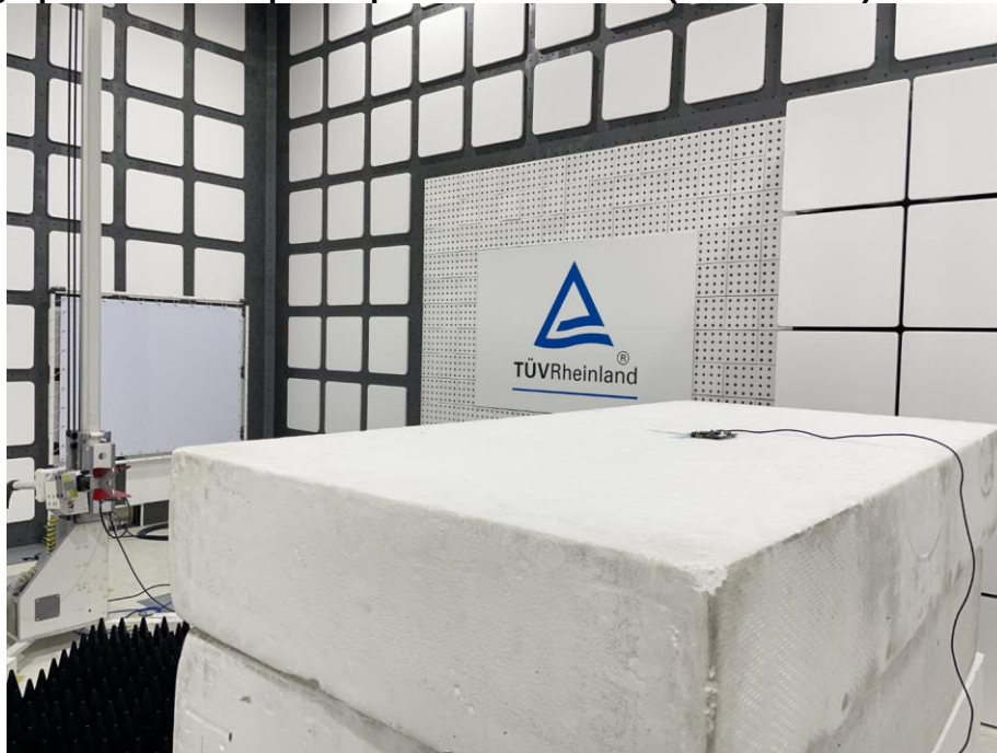
Photograph 6: Test Setup for Spurious Emissions (Back View 4)
