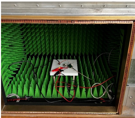
Photograph for Unwanted Emission into non-restricted frequency bands
