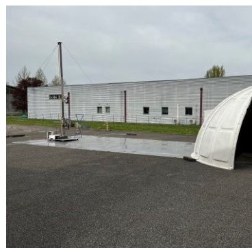
OATS Test setup (Biconic and Bi-Log antenna)
