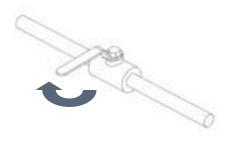
Valve should open/close easily by hand, without the use of any tools. The valve handle should be perpendicular to the pipe, which means the valve is closed.
