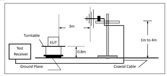
(c) For radiated emissions above 1000MHz
