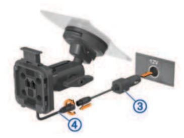
6 Tighten the collar around the connected power cables.
