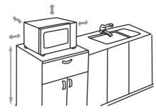
minimum clearance of 12 inches (30cm) above the oven. The minimum installation height is 36 inches(91.4cm).
