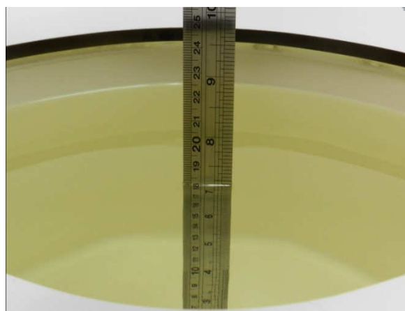
Fig 10.2 Photo of Liquid Height for Body SAR
