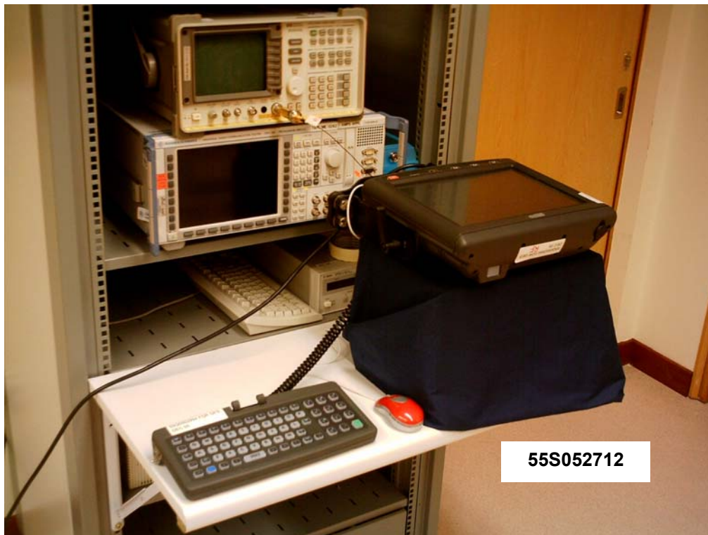
Band Edge Compliance Test Setup
