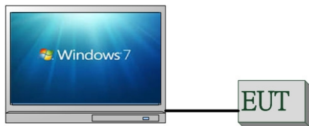
Fig.2-2 Conducted Emission (Antenna Port) Configuration
