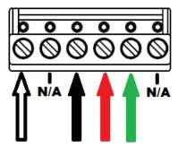
After the reader is terminated and connected on both ends and power is applied, the blue LED should turn on and the reader should be ready to use within 0 to 10 minutes (depending on system updates). THIS DEVICE COMPLIES WITH PART 15 OF THE FCC RULES. OPERATION IS SUBJECT TO THE FOLLOWING TWO CONDITIONS: (1) THIS DEVICE MAY NOT CAUSE HARMFUL INTERFERENCE, AND (2) THIS DEVICE MUST ACCEPT ANY INTERFERENCE RECEIVED, INCLUDING INTERFERENCE THAT MAY CAUSE UNDESIRED OPERATION.
