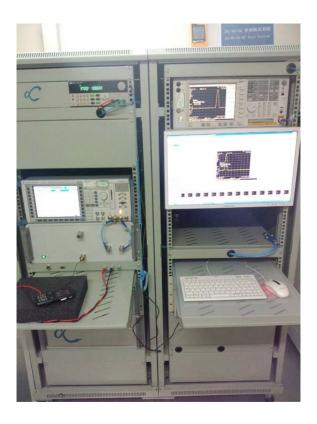
Radiated emission test setup
