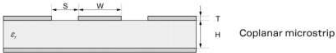
Figure 35: Coplanar microstrip dimension specification
