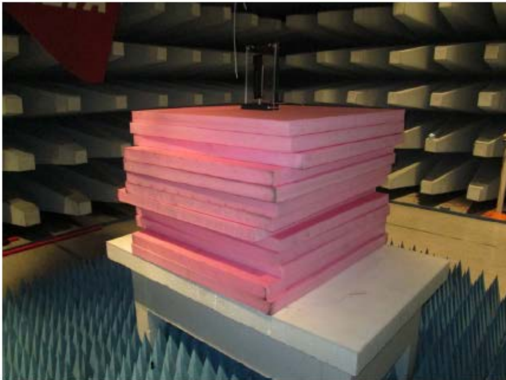
Photo 4.8.1 Test setup regarding measurement of radiated emission. 1-18 GHz.
