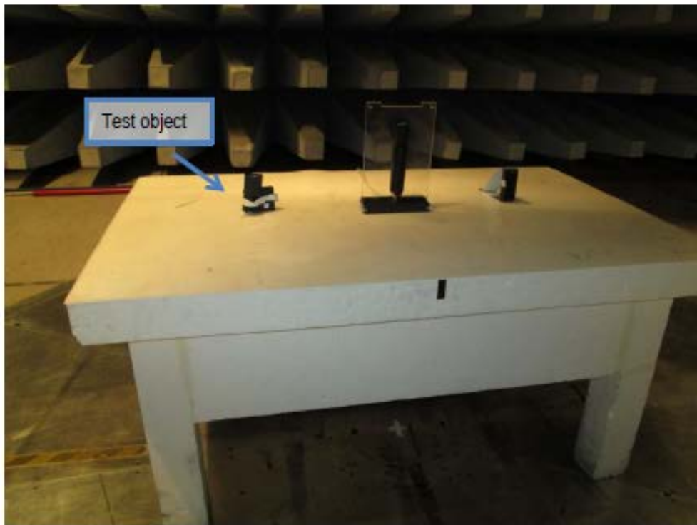
Photo 4.7.1 Test setup regarding measurement of radiated emission below 1 GHz.
