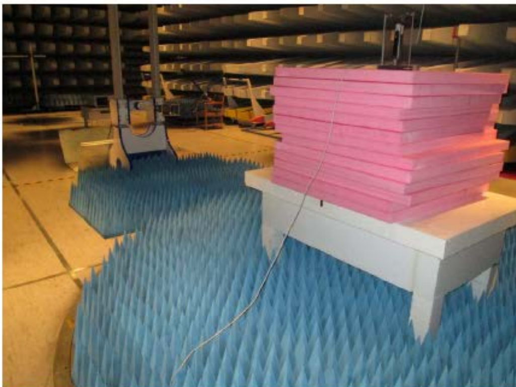
Photo 4.8.2 Test setup regarding measurement of radiated emission 1-18 GHz.
