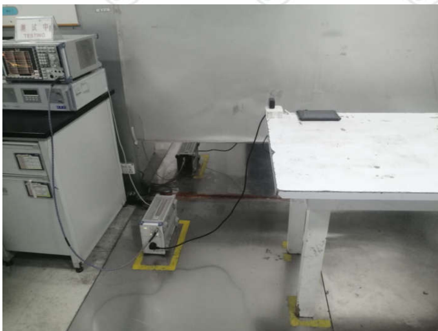
Conducted Emissions Test Setup
