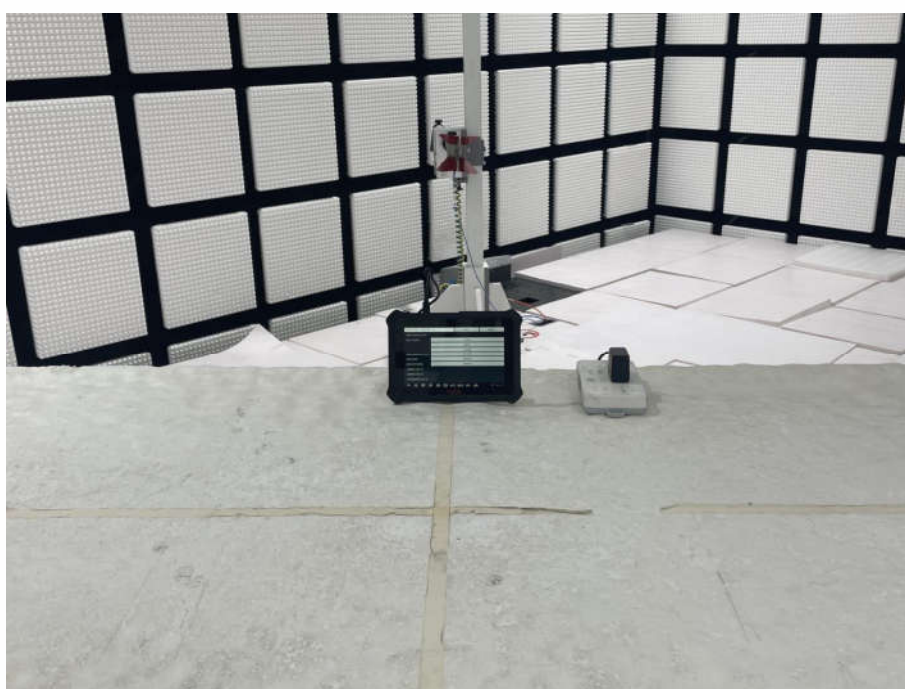
Radiated spurious emission Test Setup-2(Above 1GHz)
