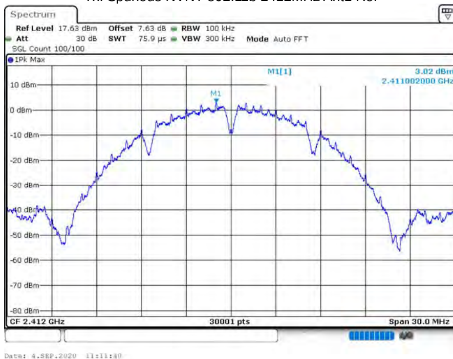
Tx. Spurious NVNT 802.11b 2412MHz Ant1 Ref
