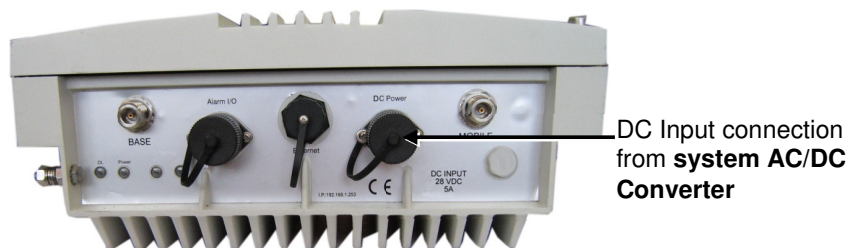
Figure 3-9. DC Power Input Connection Location
