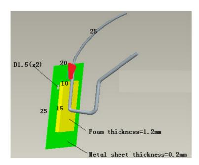
Figure 1 Physical dimension (mm)
