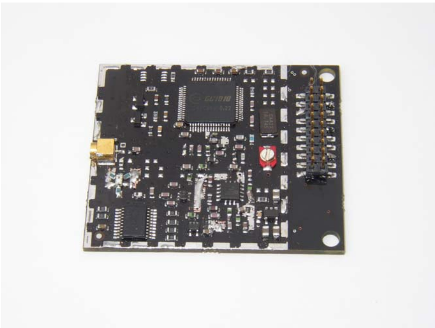
EUT – Transceiver Component View with Shield Removed
