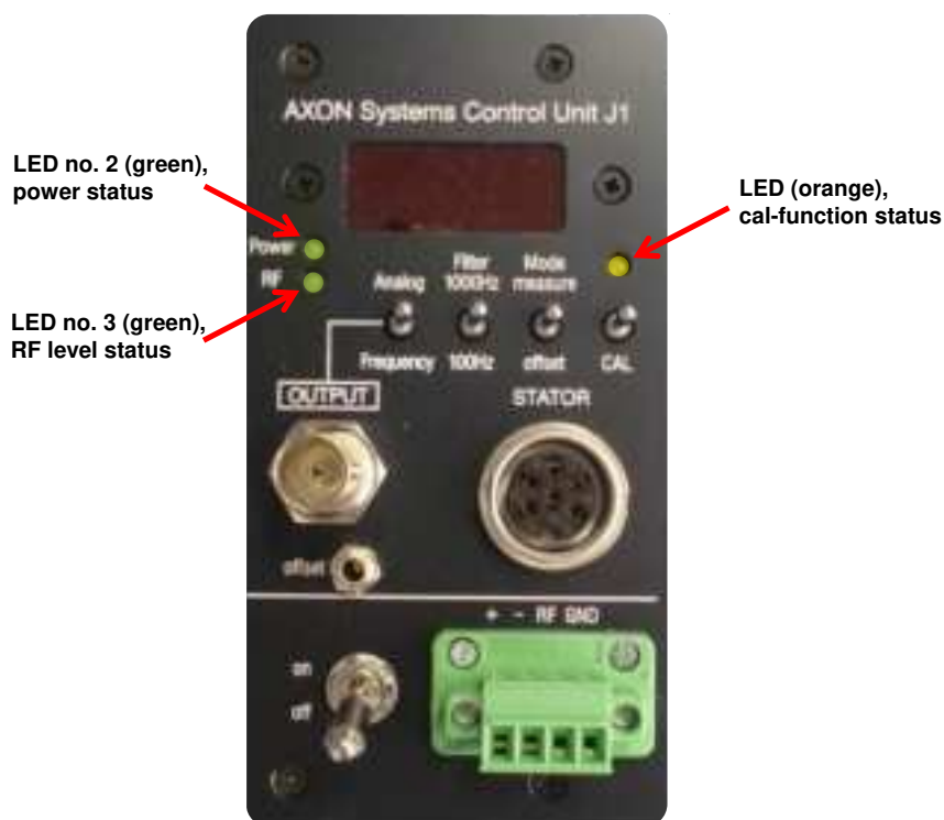
Fig. 8.1: LEDs on the evaluation unit
