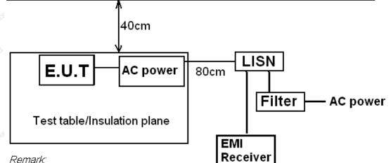
Remark: E.U.T: Equipment Under Test LISN: Line Impedence Stabilization Network Test table height=0.8m
