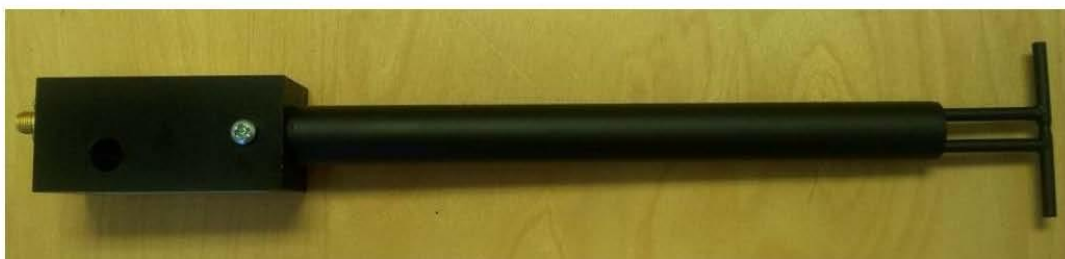
Figure 1 – MVG COMOSAR Validation Dipole
