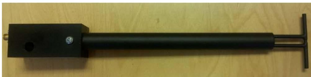
Figure 1 – MVG COMOSAR Validation Dipole
