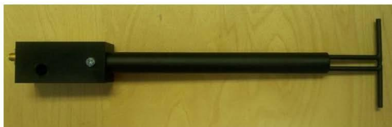
Figure 1 – MVG COMOSAR Validation Dipole
