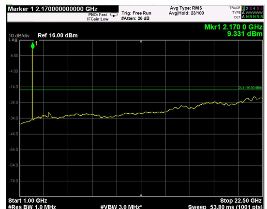
Channel: TOP, Modulation: 16QAM, BW=20MHz, Range: Upper
