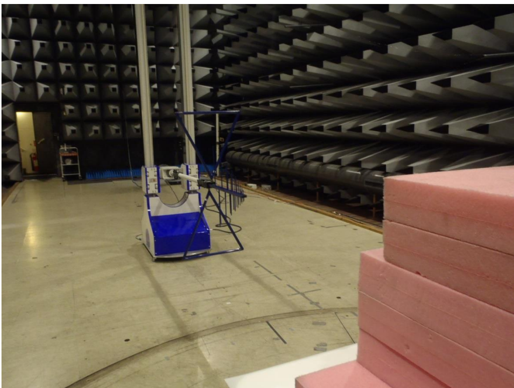
Photo 4.2.2 Test setup regarding measurement of radiated emission.
