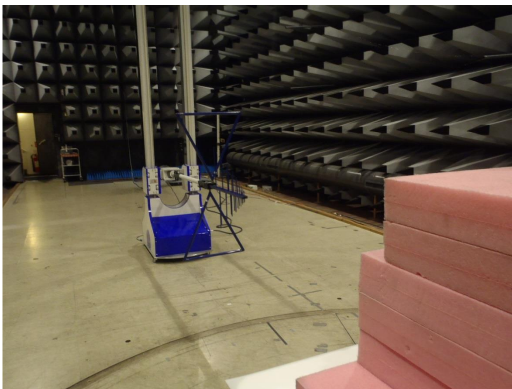
Photo 4.4.2 Test setup regarding measurement of band edge compliance.
