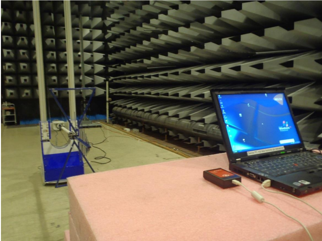
Photo 4.2.1 Test setup regarding measurement of radiated emission.
