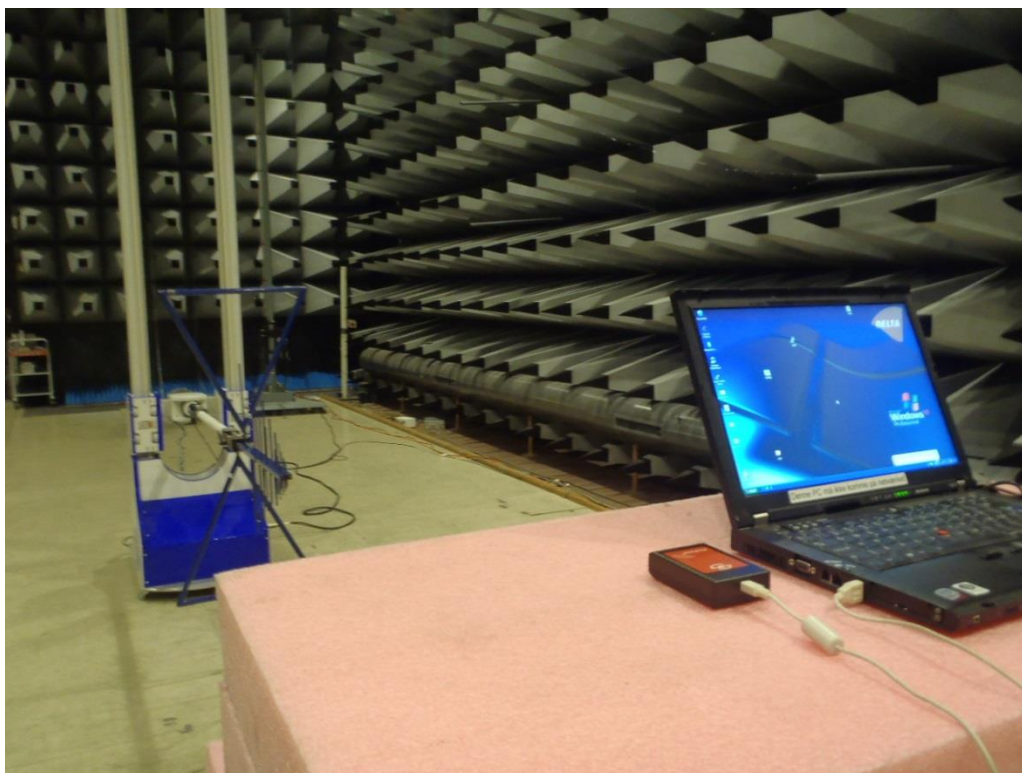
Photo 4.4.1 Test setup regarding measurement of band edge compliance.
