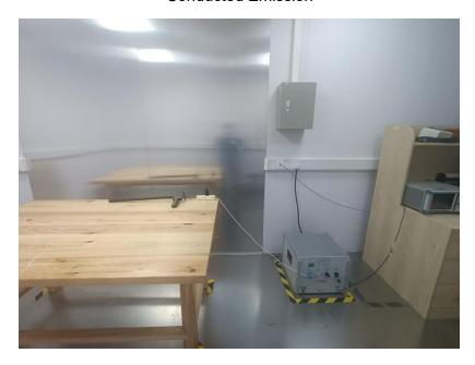
Radiated Spurious Emissions From 30MHz-1000MHz
