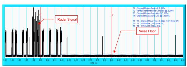
**NOTE:** An expanded plot for the device vacates the channel in the required 500ms.
