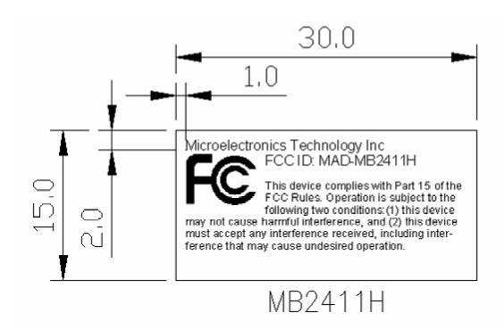
2. LETTERING: BLACK (THERMAL TRANSFER RIBBON FOR BAR CODE PRINTER).
