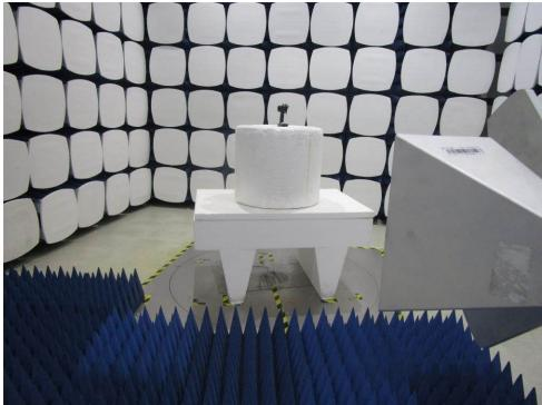
1.2 Radiated Spurious Emissions Test Setup
