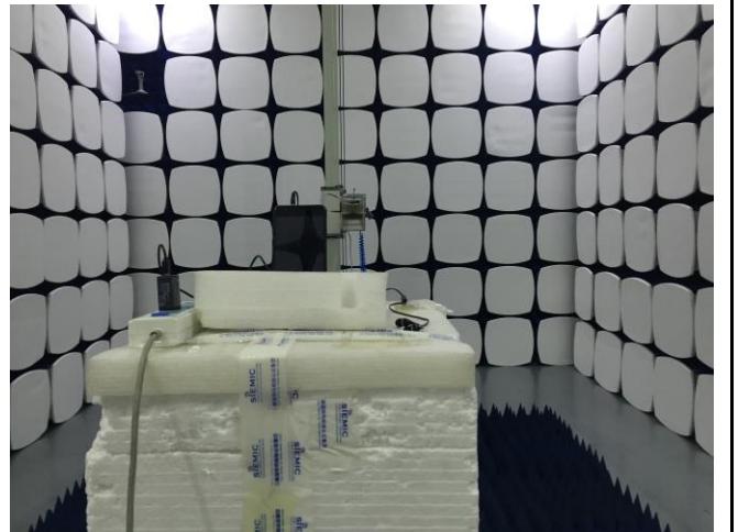
Radiated Spurious Emissions Test Setup Above 1GHz
