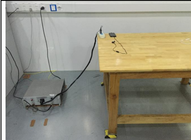
Conducted Emissions Test Setup Front View
