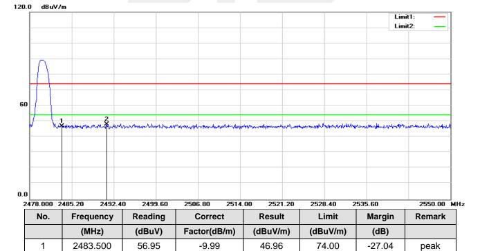
Note: GFSK,  $\pi/4$ -DQPSK,8DPSK of the nohopping and hopping mode all have been test, the worst case is GFSK of the nohopping mode, this report only show the worst case.
