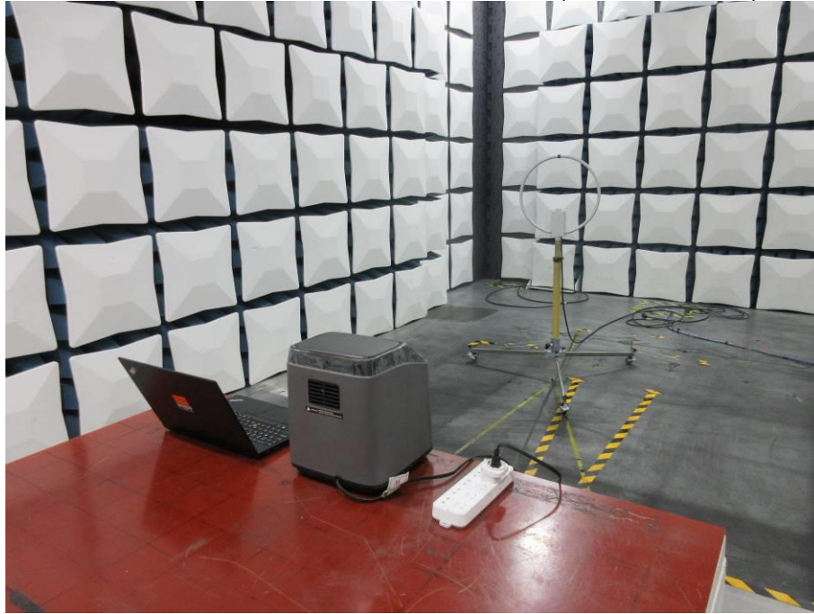
RADIATED RF MEASUREMENT SETUP (9KHz ~ 30 MHz)
