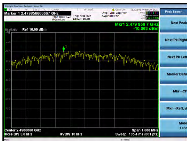
GFSK(BLE 1Mbps) HIGH CHANNEL
