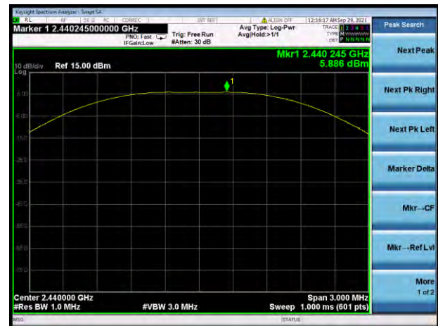
GFSK(BLE 1Mbps) MIDDLE CHANNEL
