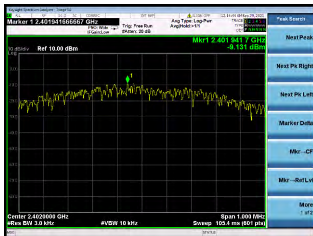
GFSK(BLE 1Mbps) LOW CHANNEL
