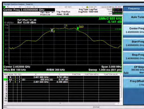
GFSK(BLE 1Mbps) LOW CHANNEL
