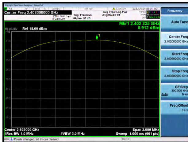
GFSK(BLE 1Mbps) LOW CHANNEL
