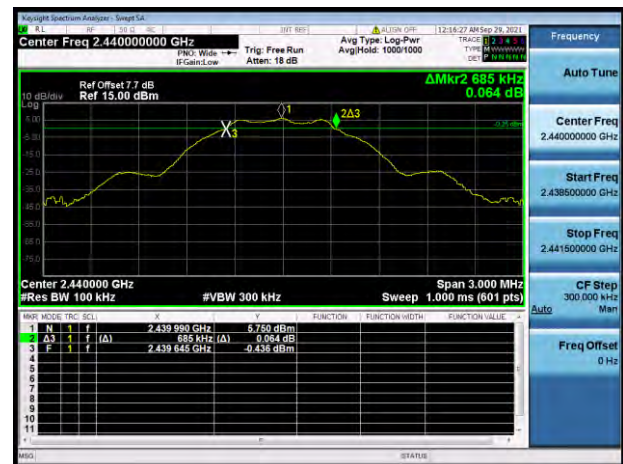
GFSK(BLE 1Mbps) MIDDLE CHANNEL
