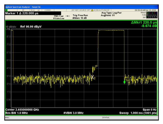
Number of Pulses in Pulse Train = 16 Time per Each Pulse = 220 us Total On Time = 3.52 ms Total Duty Cycle = 3.52 ms / 21.90 ms = 16.073% The Peak to Average Ratio is -15.87 dB
