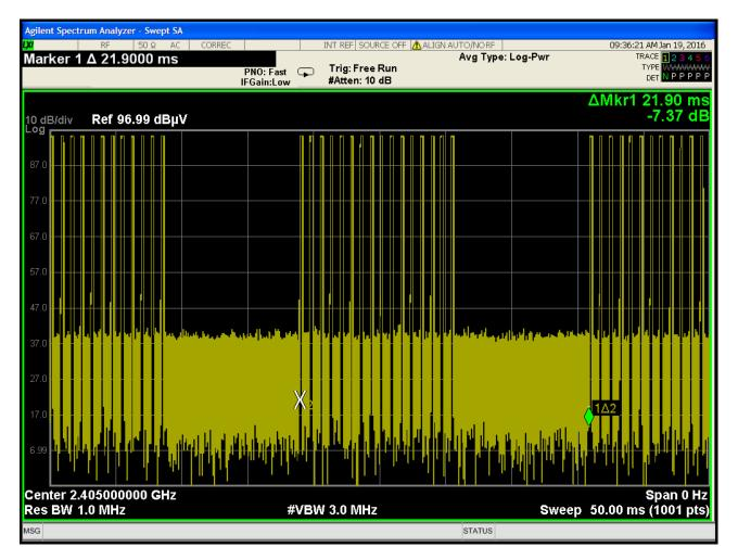
Time of One Pulse with Blanking Interval = 21.90 ms
