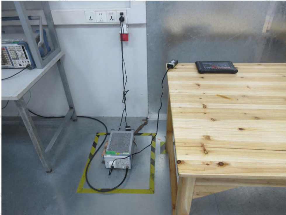
Photo of Power Line Conducted Emission Test
