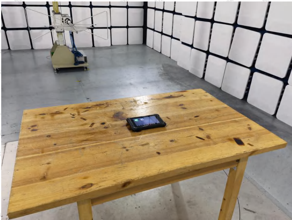
Photo of Radiation Emission Test
