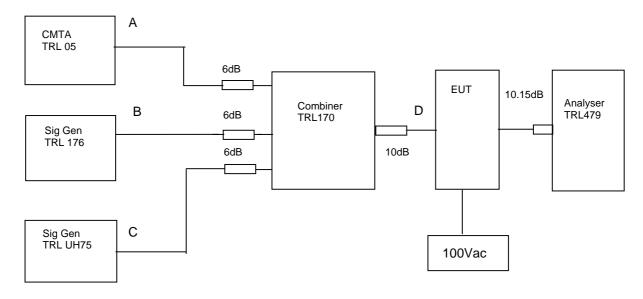
The intermodulation and spurious products were measured with the amplifier operating at maximum gain. A three tone test was conducted using the equipment as above. The input power level was adjusted so the level at point D was 10dB above the maximum input of –61.3dBm.The cable and attenuator loss between the EUT and the spectrum analyser was 10.15dB.
