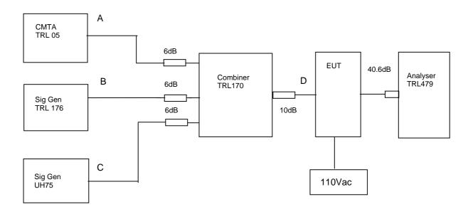
The Intermodulation and spurious products were measured with the amplifier operating at maximum gain. A three tone test was conducted using the equipment as above. The input power level was adjusted so the level at point D was 10 dB above the maximum input of -19.0dBm. The cable and attenuators loss between the EUT and the spectrum analyser was 40.6 dB.
