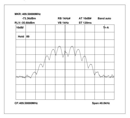
409.5 MHz Signal Generator and EUT, deviation set to 5kHz
