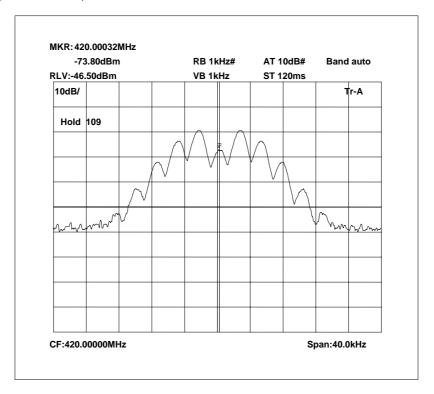
420.0 MHz Signal Generator and EUT, deviation set to 5kHz
