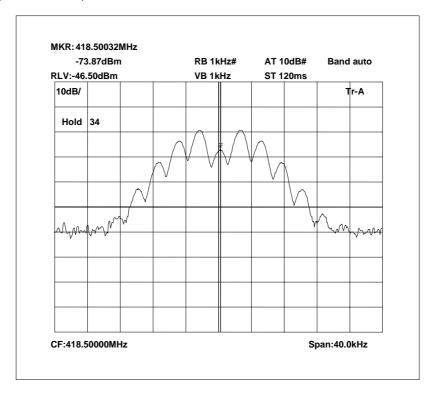
418.5 MHz Signal Generator and EUT, deviation set to 5kHz
