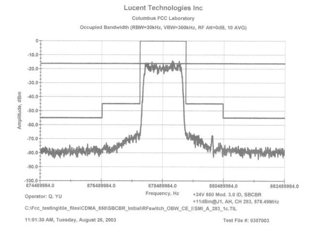
Cellular A-Band: Upper Edge Channel Channel 283, 878.49 MHz Measured at the output of SBCBR transceiver
