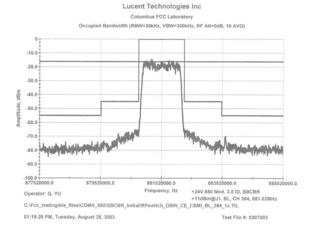
Cellular B-Band: Lower Edge Channel Channel 384, 881.52 MHz Measured at the output of SBCBR transceiver
