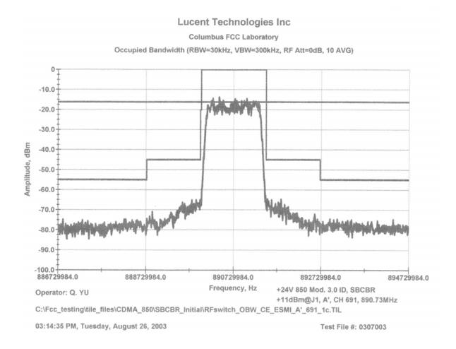
Cellular A'-Band Channel 691, 890.73 MHz Measured at the output of SBCBR transceiver
