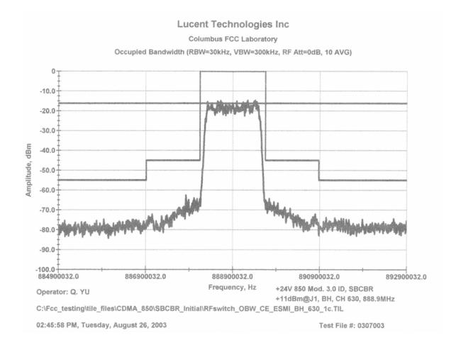
Cellular B-Band: Upper Edge Channel Channel 630, 888.9 MHz Measured at the output of SBCBR transceiver
