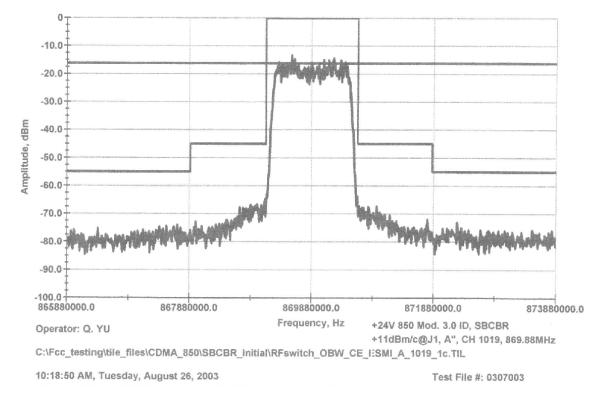
Cellular A"-Band Channel 1019, 869.88 MHz Measured at the output of SBCBR transceiver
