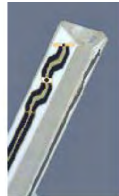
Figure 2.3 Probe Thick-Film Technique
