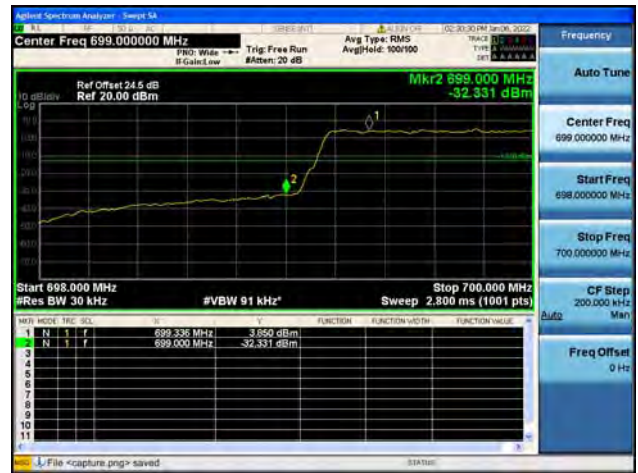
Band12 / 1.4MHz / High CH / QPSK / FULL RB
