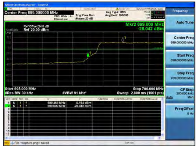
Band12 / 3MHz / High CH / QPSK / FULL RB
