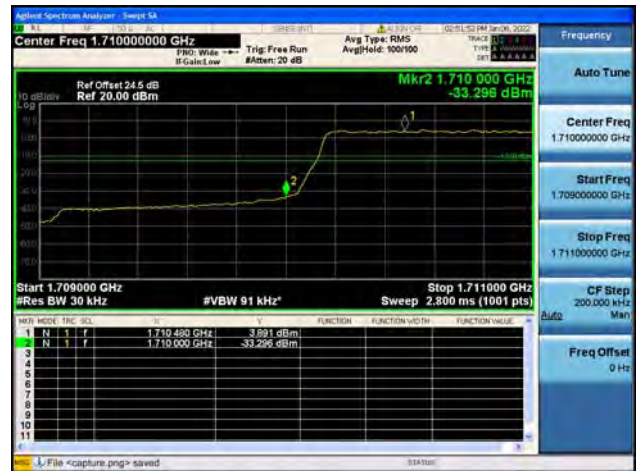
Band66 / 1.4MHz / High CH / QPSK / FULL RB
