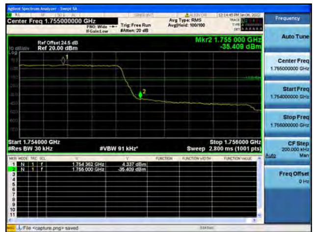
Band4 / 1.4MHz / High CH / QPSK / FULL RB
