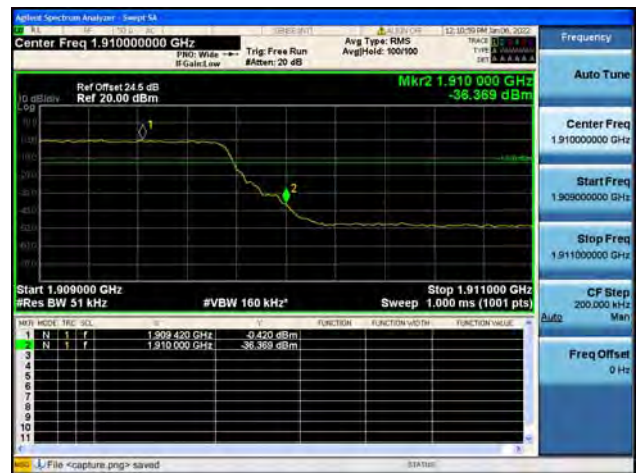
Band2 / 5MHz / High CH / QPSK / FULL RB
