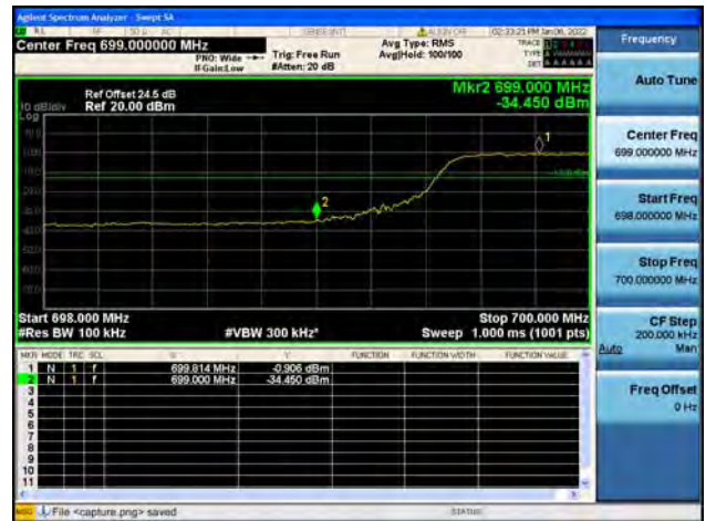
Band12 / 10MHz / High CH / QPSK / FULL RB
