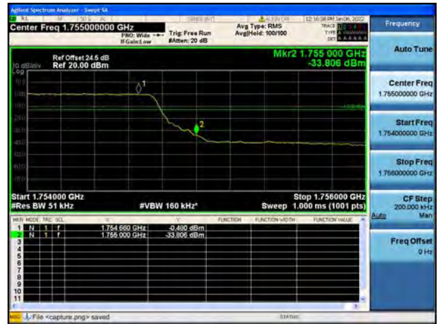
Band4 / 5MHz / High CH / QPSK / FULL RB
