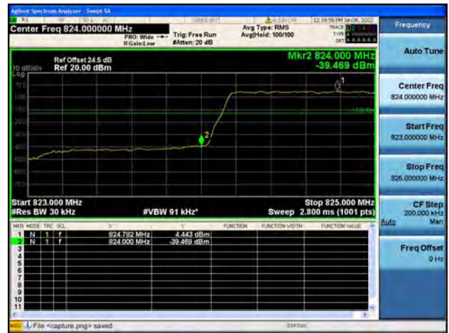
Band5 / 1.4MHz / High CH / QPSK / FULL RB
