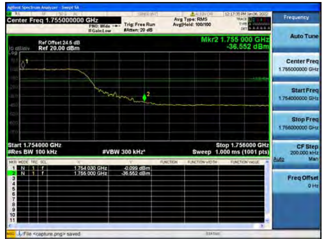
Band4 / 10MHz / High CH / QPSK / FULL RB
