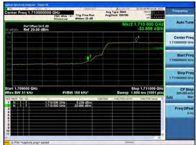
Band66 / 5MHz / High CH / QPSK / FULL RB
