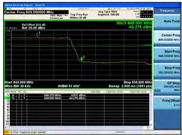
Band5 / 1.4MHz / High CH / QPSK / FULL RB
