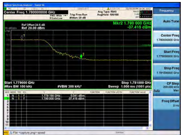
Band66 / 10MHz / High CH / QPSK / FULL RB
