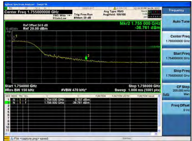
Band4 / 15MHz / High CH / QPSK / FULL RB
