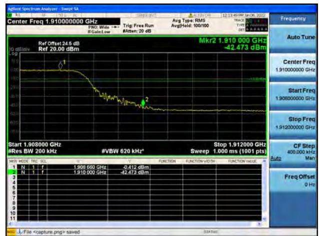
Band2 / 20MHz / High CH / QPSK / FULL RB
