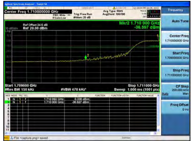
Band4 / 15MHz / High CH / QPSK / FULL RB
