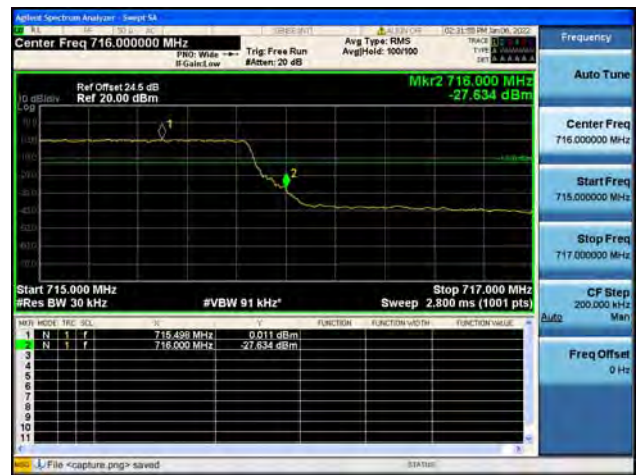
Band12 / 3MHz / High CH / QPSK / FULL RB
