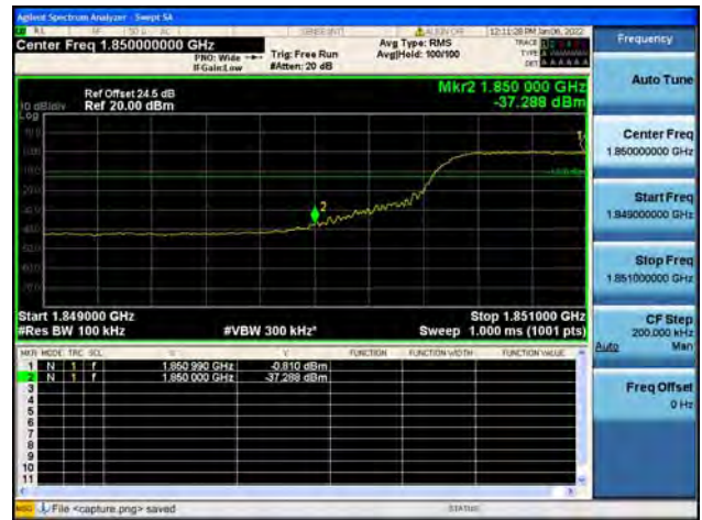
Band2 / 10MHz / High CH / QPSK / FULL RB
