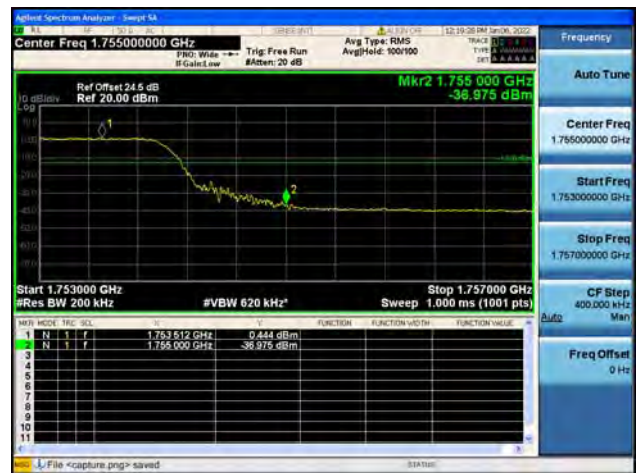
Band4 / 20MHz / High CH / QPSK / FULL RB
