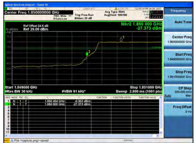
Band2 / 3MHz / High CH / QPSK / FULL RB
