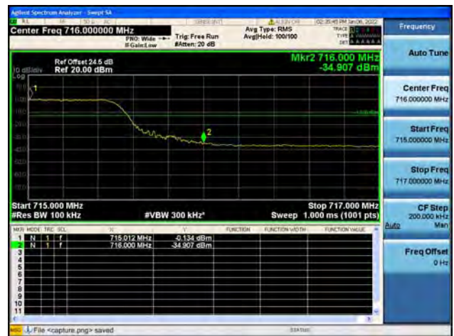
Band17 / 10MHz / High CH / QPSK / FULL RB
