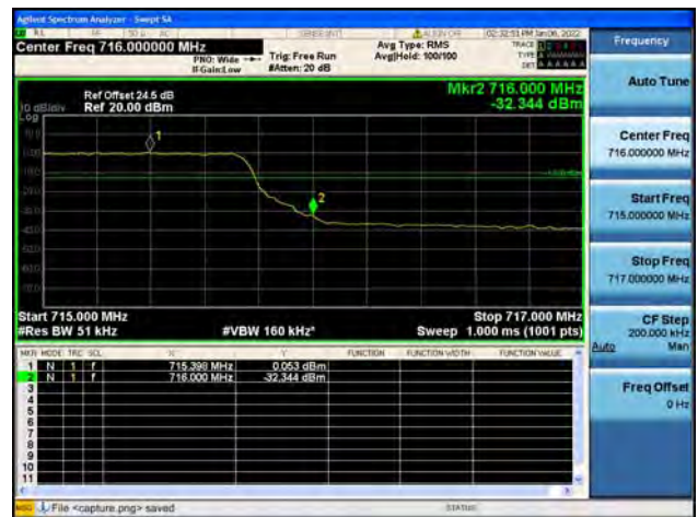
Band12 / 5MHz / High CH / QPSK / FULL RB
