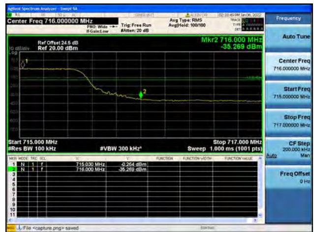
Band12 / 10MHz / High CH / QPSK / FULL RB
