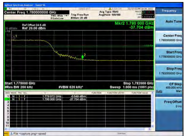
Band66 / 20MHz / High CH / QPSK / FULL RB
