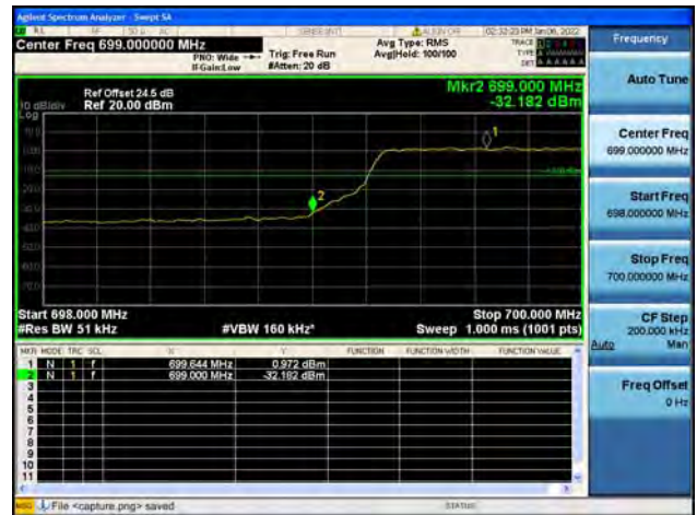
Band12 / 5MHz / High CH / QPSK / FULL RB
