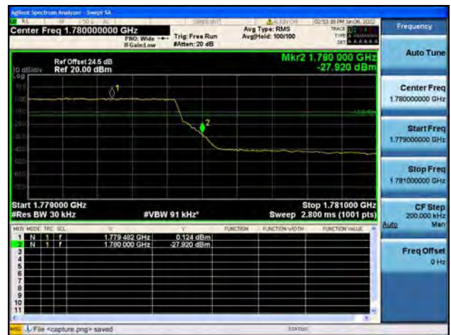
Band66 / 3MHz / High CH / QPSK / FULL RB
