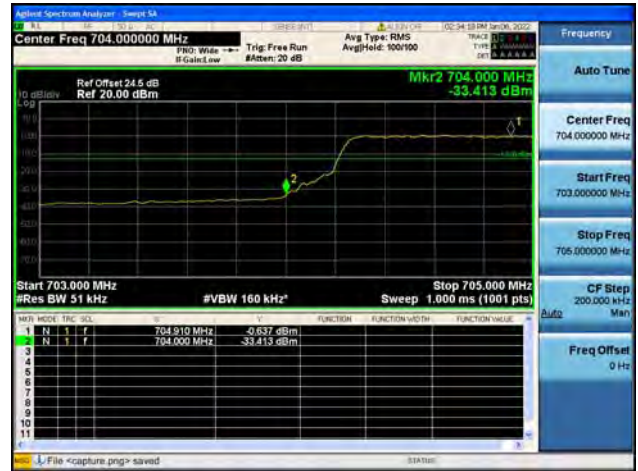
Band17 / 5MHz / High CH / QPSK / FULL RB
