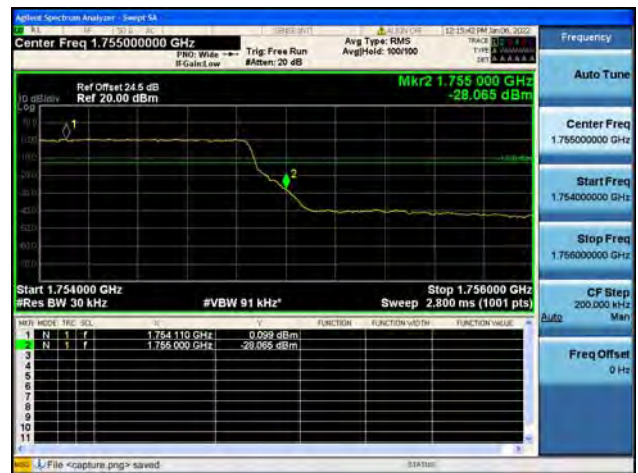
Band4 / 3MHz / High CH / QPSK / FULL RB
