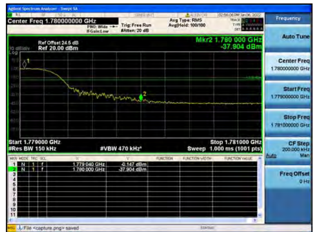
Band66 / 15MHz / High CH / QPSK / FULL RB
