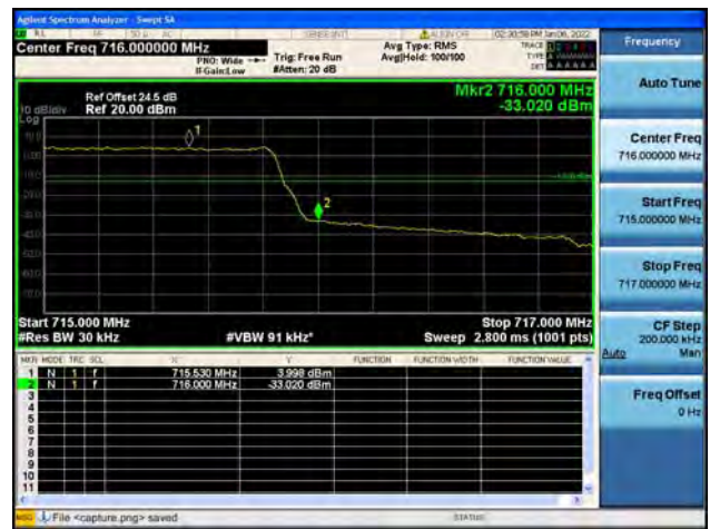
Band12 / 1.4MHz / High CH / QPSK / FULL RB
