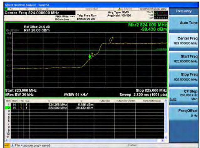
Band5 / 3MHz / High CH / QPSK / FULL RB
