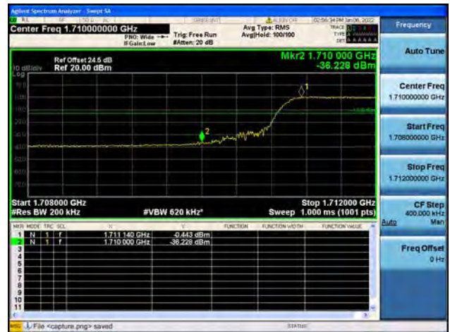
Band66 / 20MHz / High CH / QPSK / FULL RB
