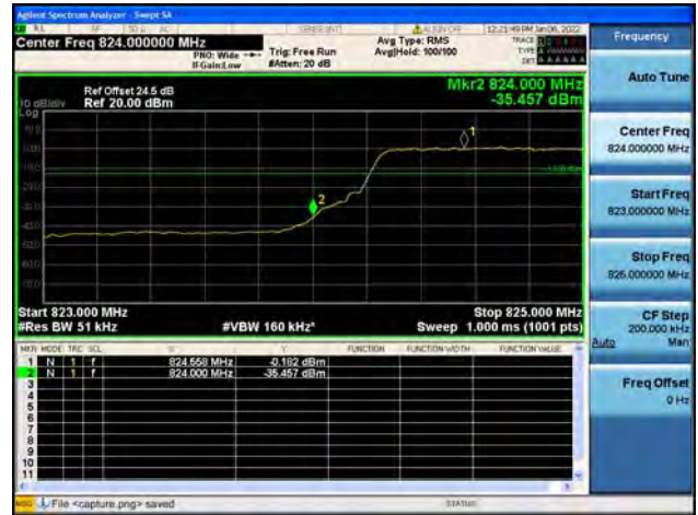
Band5 / 5MHz / High CH / QPSK / FULL RB
