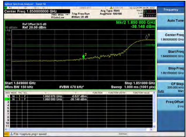
Band2 / 15MHz / High CH / QPSK / FULL RB
