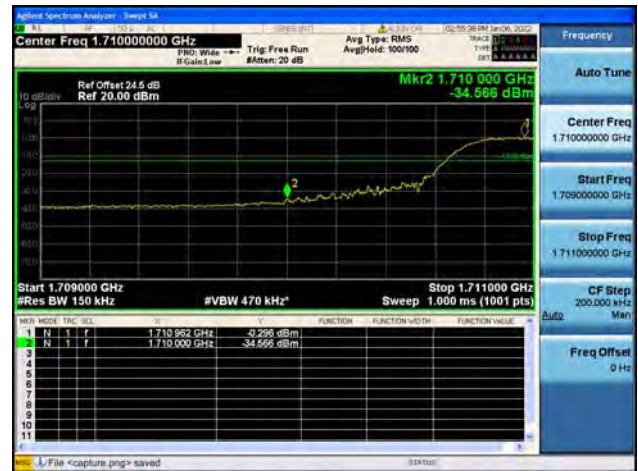
Band66 / 15MHz / High CH / QPSK / FULL RB
