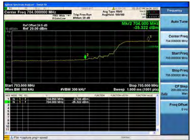
Band17 / 10MHz / High CH / QPSK / FULL RB
