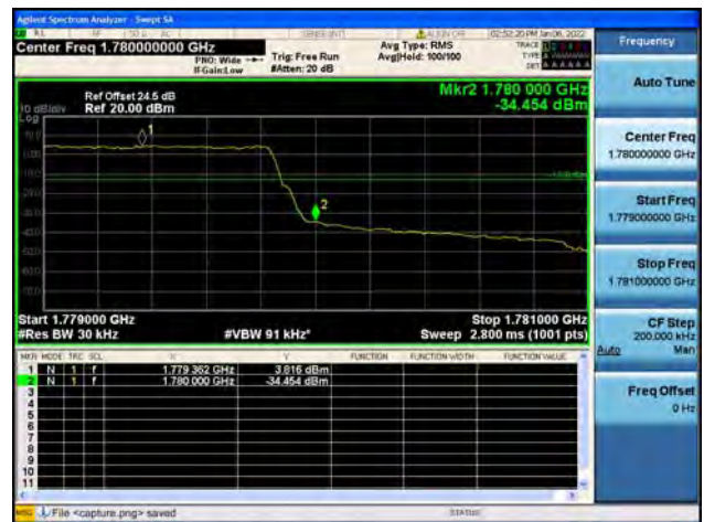
Band66 / 1.4MHz / High CH / QPSK / FULL RB
