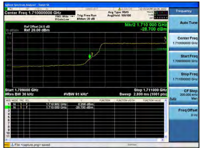
Band4 / 3MHz / High CH / QPSK / FULL RB
