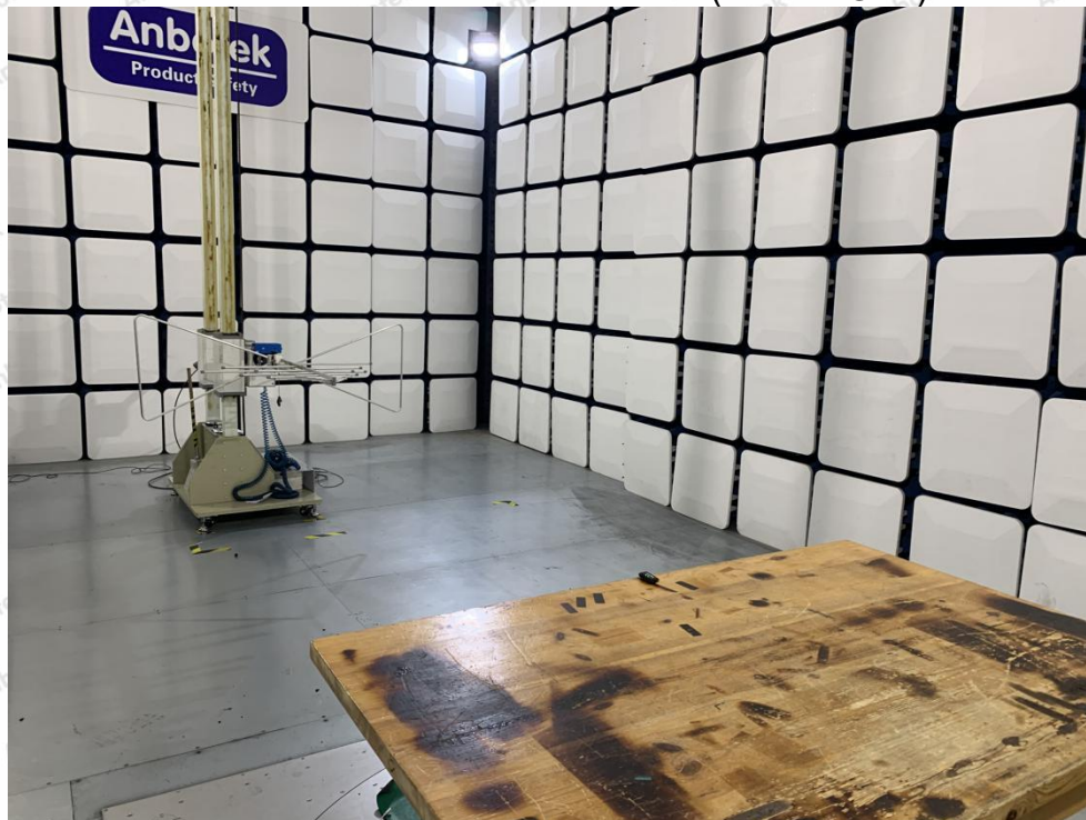
Photo of Radiation Emission Test (below 1GHz)
