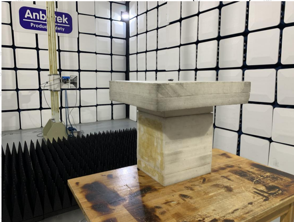
Photo of Radiation Emission Test (above 1GHz)
