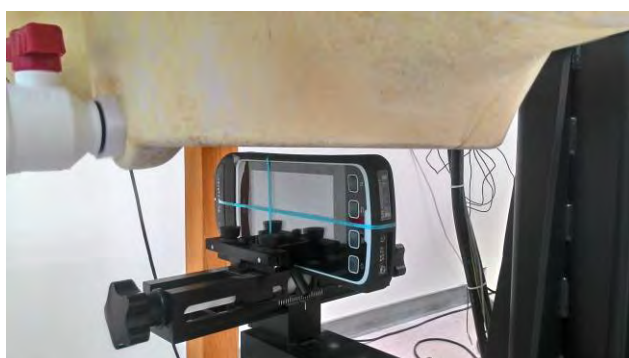
Fig.5 EUT right side to flat phantom
