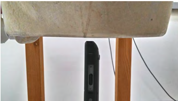
Fig.7 EUT bottom side to flat phantom
