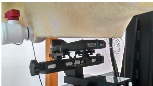
Fig.4 EUT back side to flat phantom
