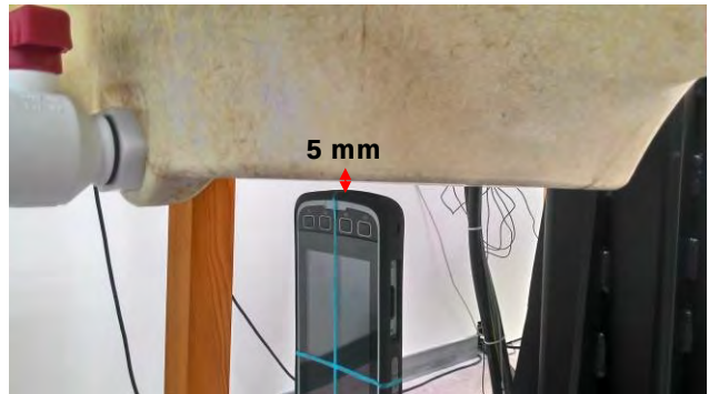
Fig.7 EUT bottom side to flat phantom
