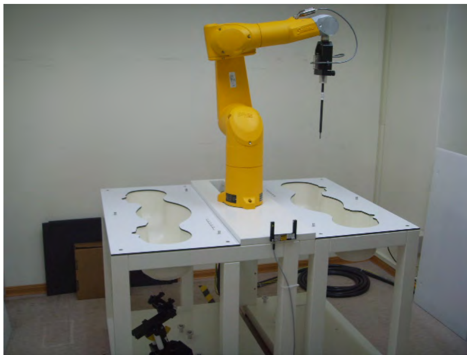
Fig.1 Photograph of the SAR measurement system
