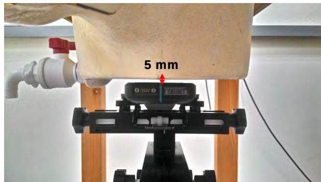
Fig.3 EUT front side to flat phantom
