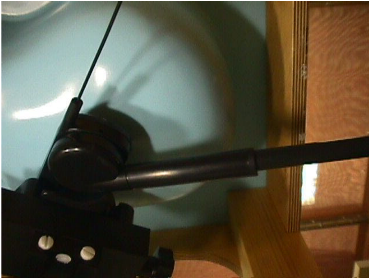
4. Globalstar Ant in Zenith Position, whip extended
