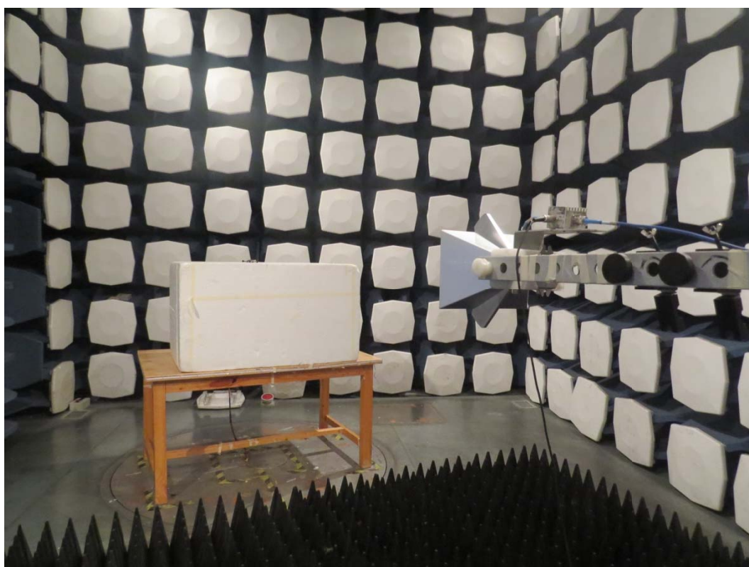
Picture 2 Radiated Spurious Emissions Test setup
