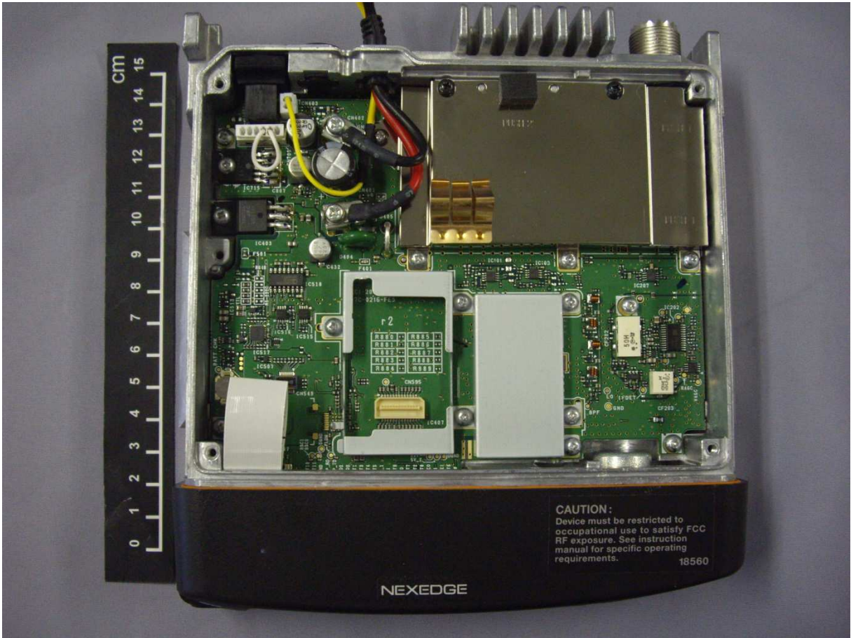
Top Internal View of Main Unit
