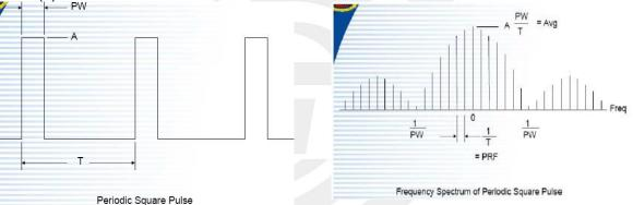
If using spectrum analyzer to measure pulse signal, it have to make sure the RBW use is at least 2/PW
