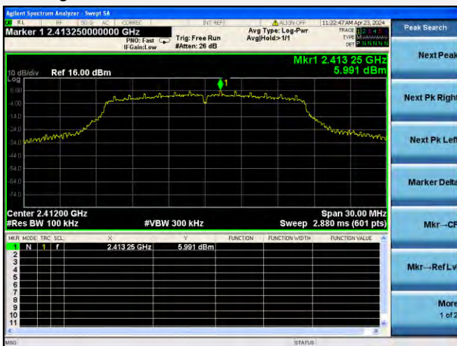
802.11g LOW CHANNEL, CARRIER LEVEL
