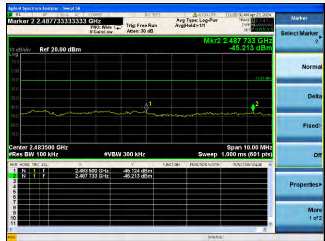
802.11b HIGH CHANNEL, BAND EDGE
