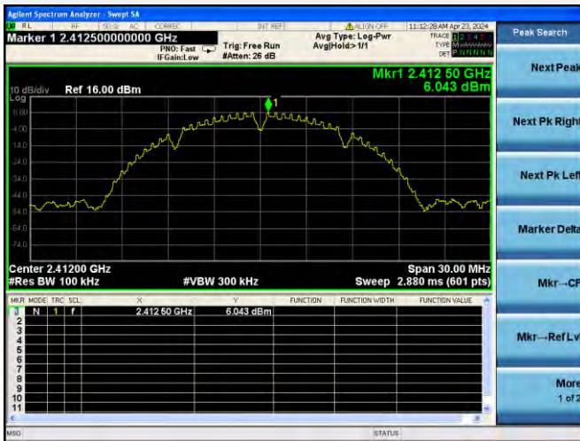
802.11b LOW CHANNEL, CARRIER LEVEL
