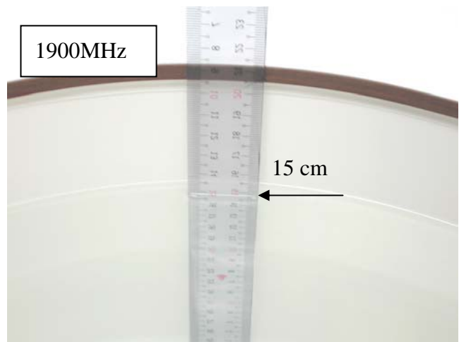
Fig.3 Photograph of the Tissue Simulant Fluid liquid depth 15cm for Flat (Body)
