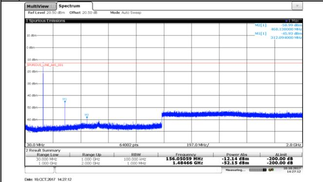
TX1 @ Test Voltage: 6V
