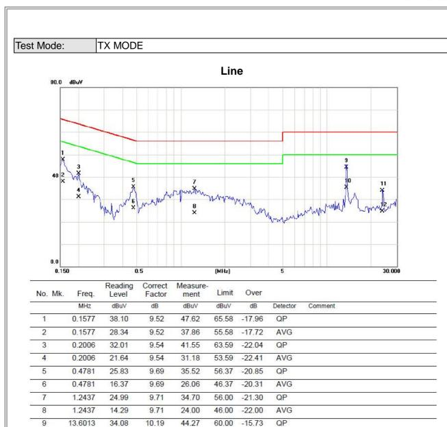
Note: The test result has included the cable loss.
