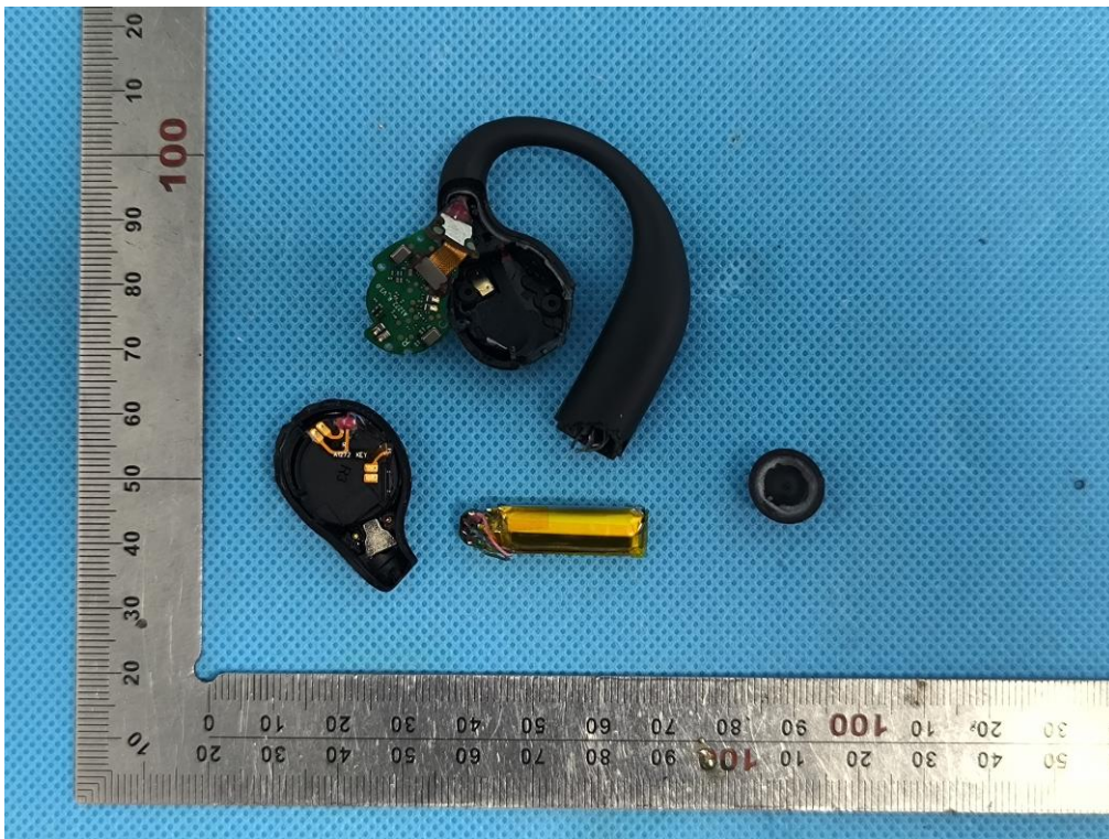
OPEN VIEW OF EUT (FIGURE 1) –WITH BATTERY HT78250VS
